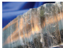
Crocidolite mineral made of amphibiole asbestos
