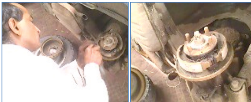
Figure 6: Asbestos brake shoe being replaced in a road side automobile repairshop
